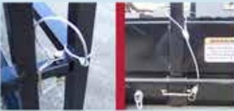
**Safety pins** are standard for all doors and side rails. Each pin is attached to the rail by a cable to prevent losing the safety pins
