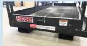
**End Fork Slots** make it easy to transport your Platform. To be used for loading and unloading only.
