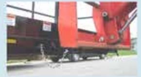
**Pins over your Fork Tines** Each pin is chained to the Platform. Fits tines up to 2 1/2" x 7 1/2". Spacing is 30" apart
